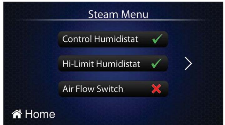
The “Steam” menu page will display the status of the four basic controls (Control Humidistat, Hi-Limit Humidistat, Air Flow Switch and Door Interlock). The humidifier will only produce steam when the unit is switched into the “ON” position, and if all four controls are satisfied.
