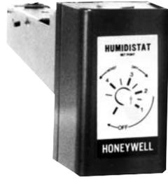
This duct mounted humidistat is installed in the return air duct to sense the humidity level in the area being served. Scale range is 15-50% RH. Differential is 4-6% non-adjustable.
