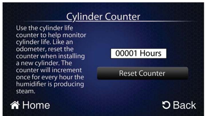
This page consists of a counter where the user can monitor the life, in hours, of the cylinder. When changing a cylinder, press the ‘Reset’ button on this page to reset the timer. The Cylinder Life Counter only counts the amount of actual runtime of the cylinder (the time when the contactor is pulled in). The counter value is saved even when the humidifier is powered down. The national average cylinder life is about 1150 hours, but this can vary greatly depending on individual water conditions.
