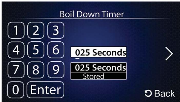
This page is where the Boil Down Timer is set. The Boil Down Timer is variable between 0 and 255 seconds, with a default value of 25 seconds. Setting the Boil Down Timer higher will result in an increased water level, and less-conditioned water. This may be helpful in reducing low water level induced arcing and corrosion of cylinders. More water is consumed by the humidifier when the Boil Down Timer value is increased.
