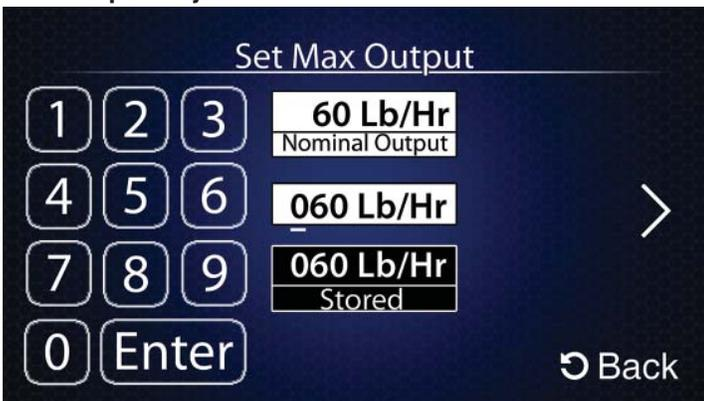
The maximum steam output of the unit can be set on this page. The maximum output value cannot exceed the nominal output value of the unit, and it cannot be set below 20% of the nominal output. The nominal output of the unit is listed on the nameplate and the previous screen.
