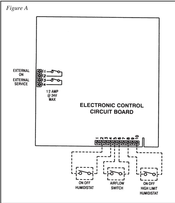
Connections shown in Figure A are for typical on-off controls. For Carnes proportional controls see the diagram below. Models HXHAG and HXHAH cannot be used with this circuit board.
