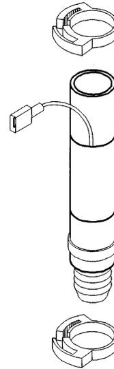
This kit contains one Circuit Board H-998-8020 (shown above), one Overflow Sensor Tube H-690-1356, and two Hose Clamps H-999-7165 (shown at right).
