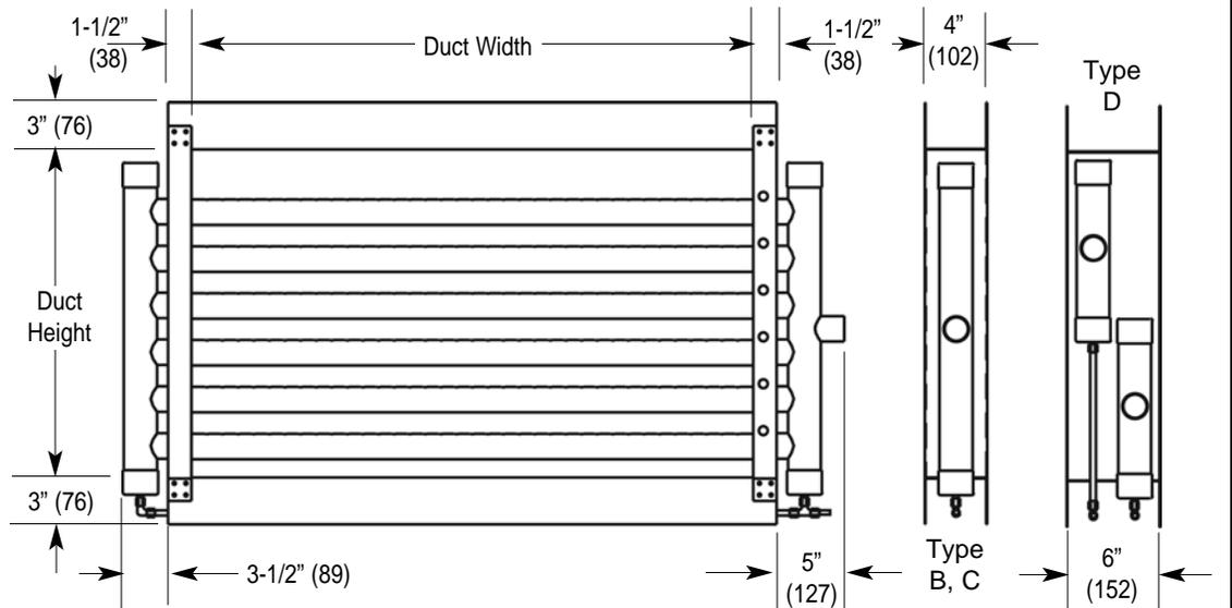
**CARNES STEAM MANIFOLDS with strong galvanized flanged frames are factory assembled to reduce installation costs.**
