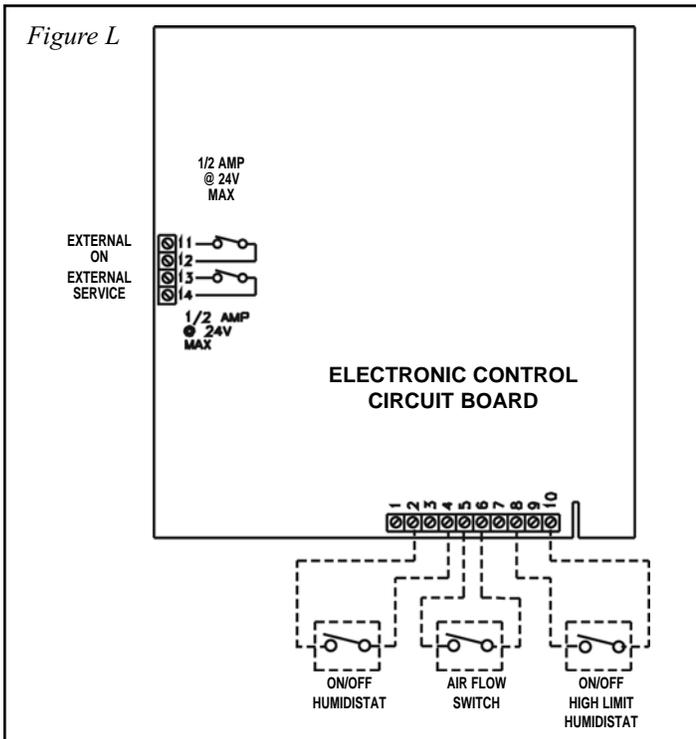
Connections shown in *Figure L* are for typical on-off controls. For Carnes proportional controls see the diagram *Figure M*. All controls are shipped with detailed wiring instructions.
