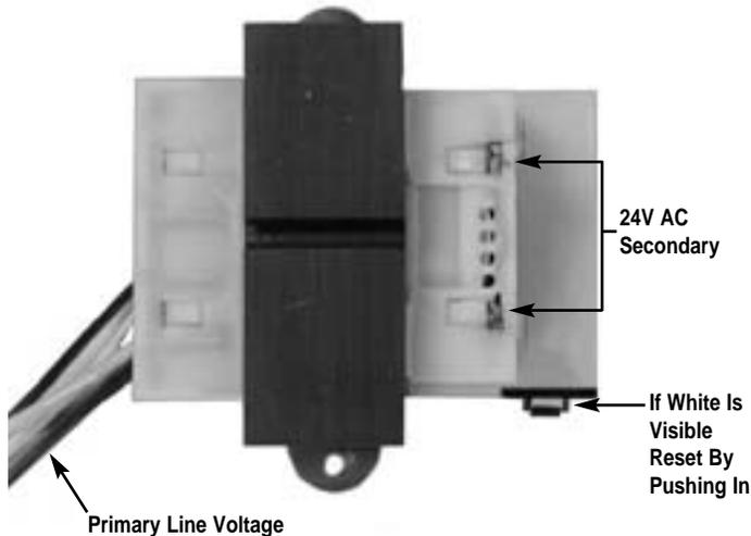
6. If 24V AC is present the electronic control board may be defective.
