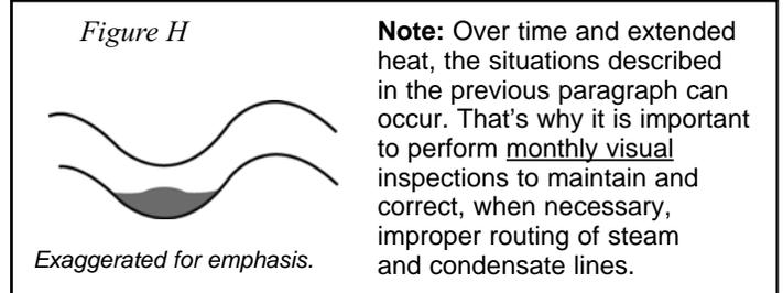
**Note:** Over time and extended heat, the situations described in the previous paragraph can occur. That's why it is important to perform monthly visual inspections to maintain and correct, when necessary, improper routing of steam and condensate lines.
