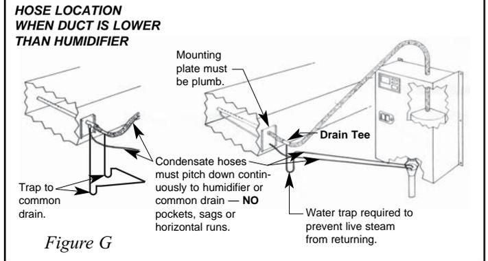
It is very important that both the steam hose and condensate return line, whether flexible or hard tubing, be installed so there are no sags, low points, dips or horizontal runs. The steam is at a very low pressure and it cannot overcome any resistance caused by accumulating water standing in the steam hose. Accumulation in the condensate return hose will hamper the flow and may cause water to enter the duct work by way of back up in distributor pipe.
