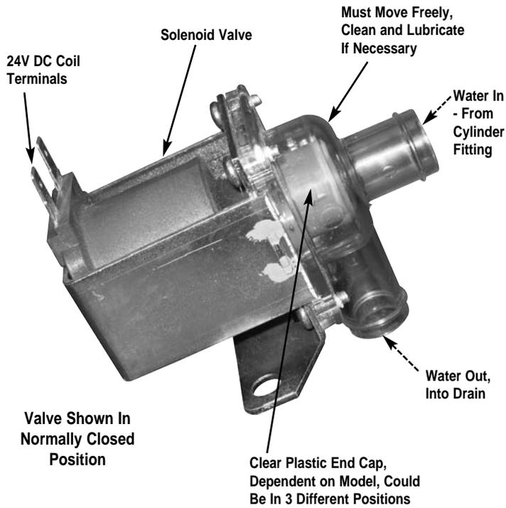
3. The “Drain Solenoid” LED indicates if the electronic circuit board is sending 24V DC to the valve. If the LED is off but 24V DC is present at the drain solenoid coil the circuit board may be defective.
