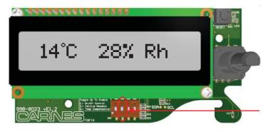
The second *(middle)* adjustable switch controls whether the unit displays its temperature reading in Celsius or Fahrenheit. If the switch is high (on), the humidistat will display Celsius. If it is low (off), the humidistat will display Fahrenheit.
