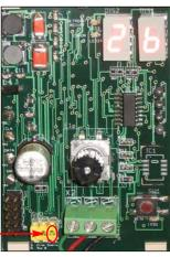
The third (farthest right) adjustable switch controls whether the two seven segment LED displays humidity or temperature when not in setpoint adjustment mode. If the switch is on, the unit displays temperature (in Fahrenheit). If the switch is off, the unit displays humidity (in % RH). If the switch is on, and the temperature being sensed is 100 degrees or greater, any digits beyond the 1's and 10's digit will not be displayed.
