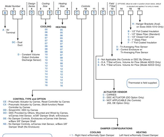
NOTE: Hand of controls is determined by facing the averaging flow sensor (inlet of the unit) with the supply air hitting the back of your head.
