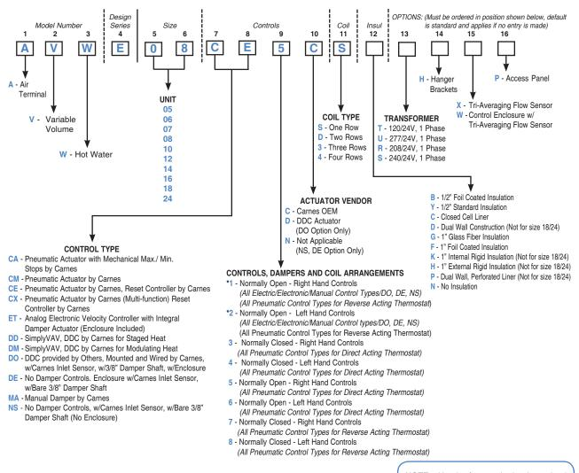
\* Electric, Electronic and DDC Units **DO NOT** fail open. '1' or '2' is used for Right or Left Hand Only. Electric/Electronic Units are shipped with the Damper in the Open Position. NOTE: Hand of controls is determined by facing the averaging flow sensor (inlet of the unit) with the supply air hitting the back of your head.
