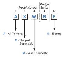
A Carnes Electric Thermostat **must be ordered** with the Electric EA and EB Control Options.
