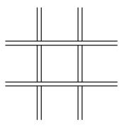
**Option D** - 3/4" round bar vertical on 6" centers through horizontal bars (3/8" x 2-1/2") on 12" centers. All intersections are welded.
