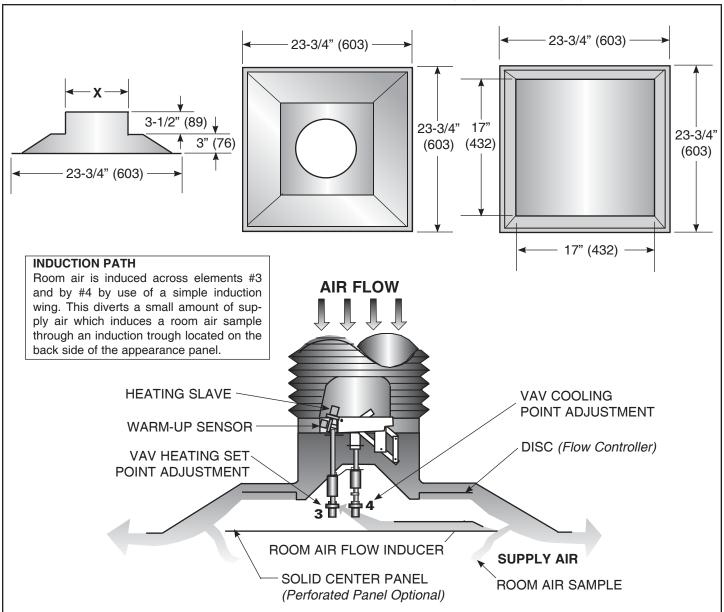
The Model SFPV/SHPV VAV provides room temperature control for heating and cooling. Separately adjustable heating and cooling set-points. Factory room temperature set-points of 74 degrees.
